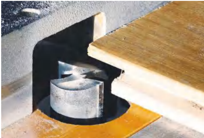
▲ Pic.5 Cleaning up the rebate on the router table using the large cutter
